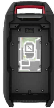
Figure 1-12 : Connexion satellite installée
