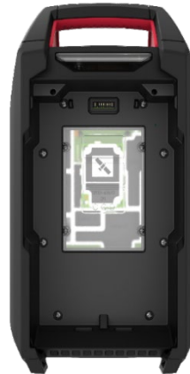
Figure 3-2: Satellite Connection Installed
